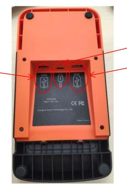
Type C interface, with P2PRO charging cable and adapter connected to the power supply to charge P2PRO.
