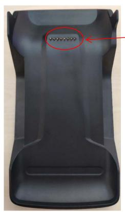
The P2 PRO sensor head needs to be aligned with the PIN connector for charging and data transmission.
